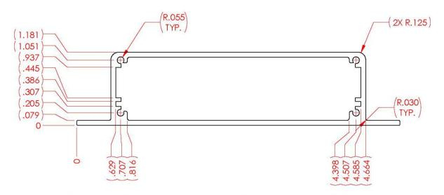
\*\*SEE DRAWING 14101615196\_001 FOR EXTRUSION DIMENSIONS & TOLERANCING\*\*
